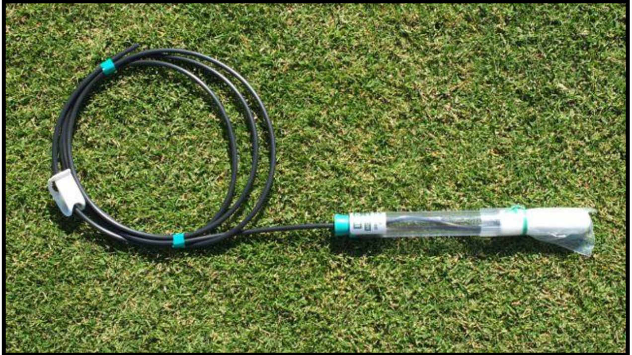
Figure 1. Suction lysimeters (Irrometer, Riverside, CA) used to capture leachate for analysis of EC L . Lysimeters were buried 4 inches below the turf surface all replicate plots for each treatment in the salinity alleviation study.
